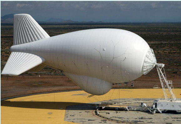
TARS uses balloons moored at about 10,000 ft as radar platforms to monitor suspicious air traffic along the southern border.
