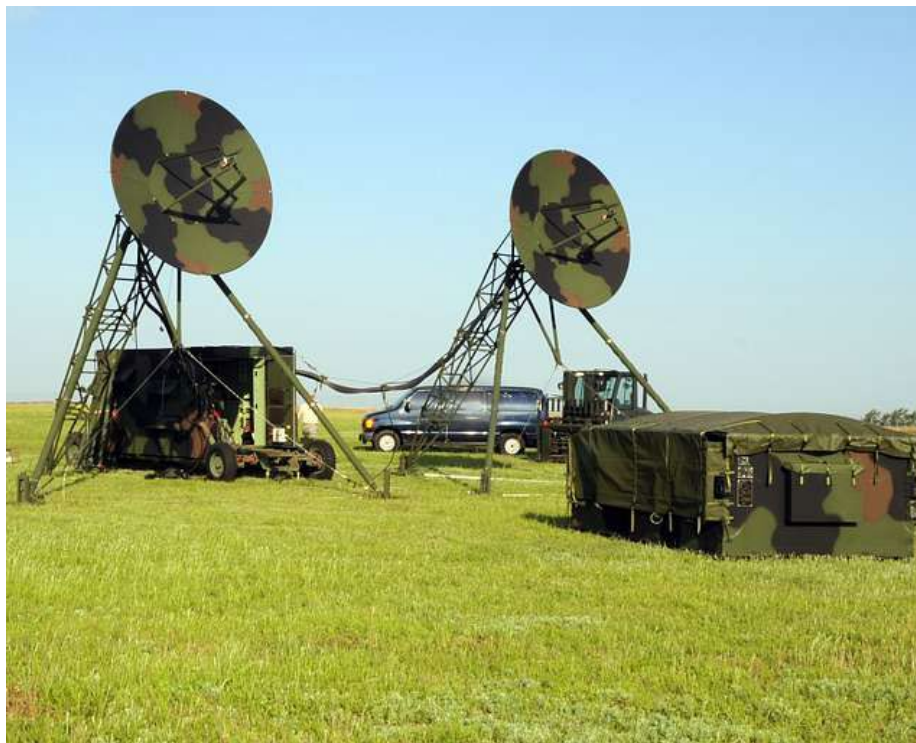
The portable Tropospheric Scatter Microwave Radio Terminal (TRC-170) can bounce microwaves off the troposphere to provide long-range voice and data links beyond the line of sight.
