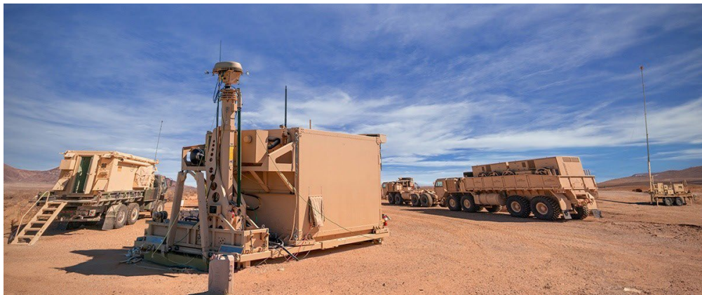
The Integrated Battle Command System combines data from various sensors and radars across the battlefield and transmits composite intelligence to warfighters. It's use in the U.S. is for training purposes. The 4 GHz antenna is at far right.
